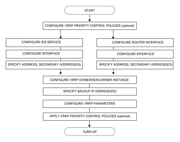
Figure 14: VRRP Configuration and Implementation Flow
